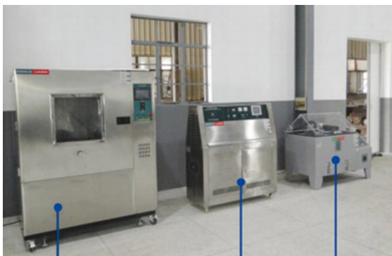
1. Rainfall Test Machine
